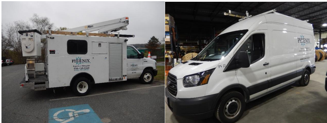
Above: Splice and Bucket truck (left), Service van (right)
